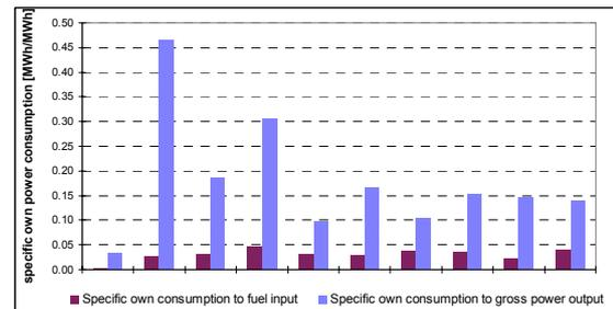
Figure 5: Own power consumption compared to fuel input and gross power output.
