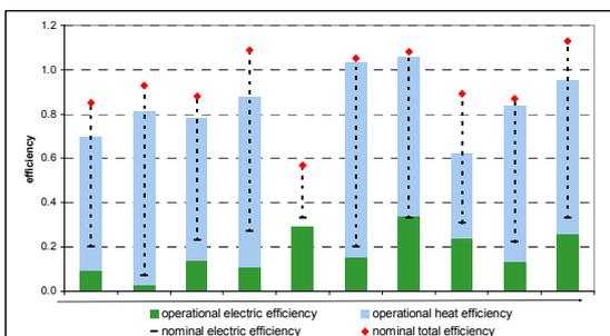
Figure 3: Nominal efficiency vs operational efficiency for individual plants.
