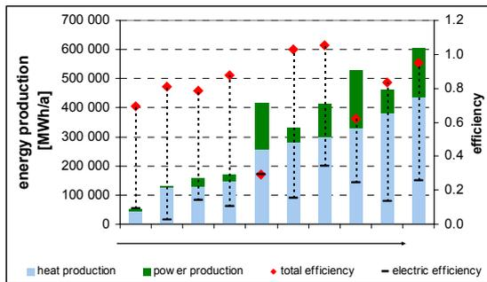
Figure 2: Annual operational efficiency and energy production for individual plants
